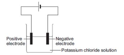
The student expected to see potassium metal at the negative electrode, but instead saw bubbles of a gas.
